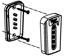
Snap open the Wireless Keyless Entry case with a coin.
